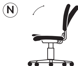
N SYNCHRO-TILT - seat and back tilt together at a 2-1 ratio. For every 2 degrees of back recline, the seat tilts 1 degree
