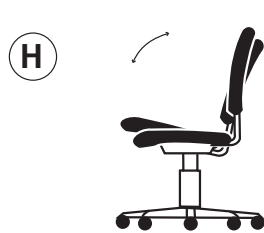
H Seat & Back Multi-tilt - seat and back tilt together at the same angle
