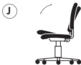
J Adjustable Tilt - Tension Control - tension of seat can be increased or decreased as desired
