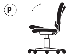
P Tilt Lock Control - seat and back tilt together locking in forward position
