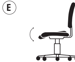
E Forward Tilt Seat Control - allows 6 degrees forward seat tilt when activated
