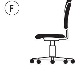
F Back Height Adjustment Control - chair back can be adjusted up and down for variable back height
