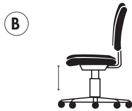
B Pneumatic Seat Height Control - seat height can be increased or decreased
